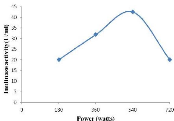
**Figure 3.** Effect of microwave power on the extraction of inulin
